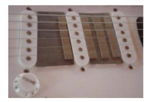
This image is the key to how the whole thing works because the electrical signal is generated right here by the electro-magnetic interaction of the magnets and strings. The rest of the invention is all
